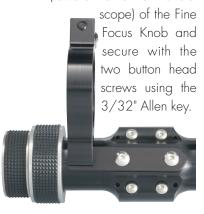
Step 3) Slip the Motor into the Motor Bracket so it is snug but still can rotate. The Drive Wheel should now be in-line with the fine focus knob of the Focusmate. Rotate the Motor until the O-rings make contact with fine focus knob.
